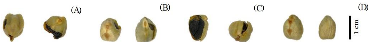
Figure 4 - Damage in chickpea seeds shown by iodine staining, due to: insects (A), seed coat rupture (B) and breakage (C); undamaged seed (D)
