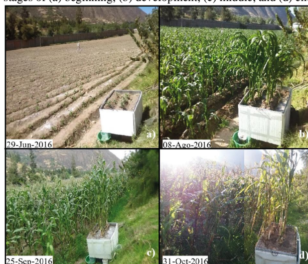
Figure 4 - Temporal variation of starchy corn phenology in the experimental plot (Parc) and drainage lysimeter (Lis) at the stages of (a) beginning, (b) development, (c) middle, and (d) end
